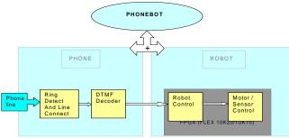
Figure 2: PHONEBOT – Basic Block Diagram
